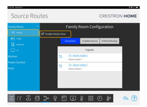
11 - Select the sources to be assigned as the input sources. Then select the device to be used to display on the outputs list. Sources should be added beforehand to the room where the driver is installed.
